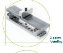
4 point bending or orcking anvil fixture for modulus of rupture Adjustable in 1 inch intervals
