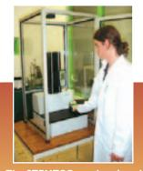
The STENTOR can be placed in a closed cabinet if sample rupture presents a risk for the operator. In that case, the motor stops as soon as the cabinet door is opened.
