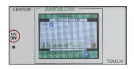
Plot the curve of your test directly on the color touch screen table top, force versus time or force versus deflection
