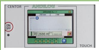
The Centor Star Touch screen is reversible without disassembly the gauge. It is possible to rotate by 90°, 180° or 270°.
