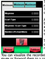
The Centor Star Touch has an internal memory that can record up to 1,000 results (maximum, minimum, calculations).
