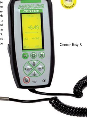
Statistics feature with automatic calculation of the avergae and standard deviation on hte 100 values in the memory.
