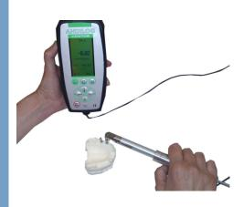
The IMPLANTORK measuring solution is used to qualify implant, tightening torque value and tightening process for the application of implant dentistry and in orthopedic surgery that require tightening or loosening.
