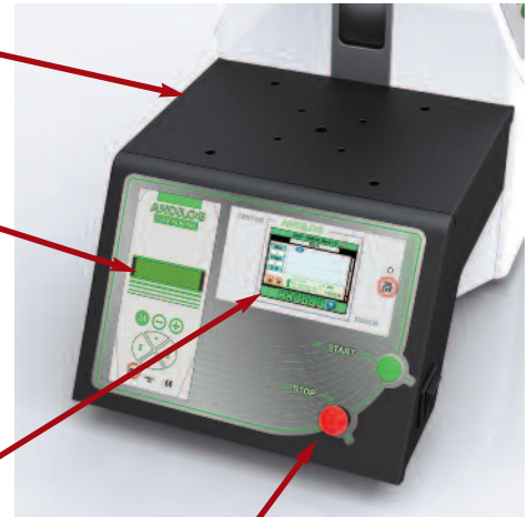
Separate control panel to setup the displacement of the test stand
