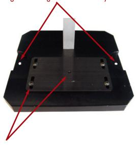
The frame base has an adjustable plate in order to align samples and force sensor (M5 female thread)
