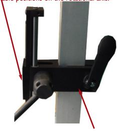
Adjusting the original height of the force gauge is done using the quick positioning cam handle, no tool is required.
