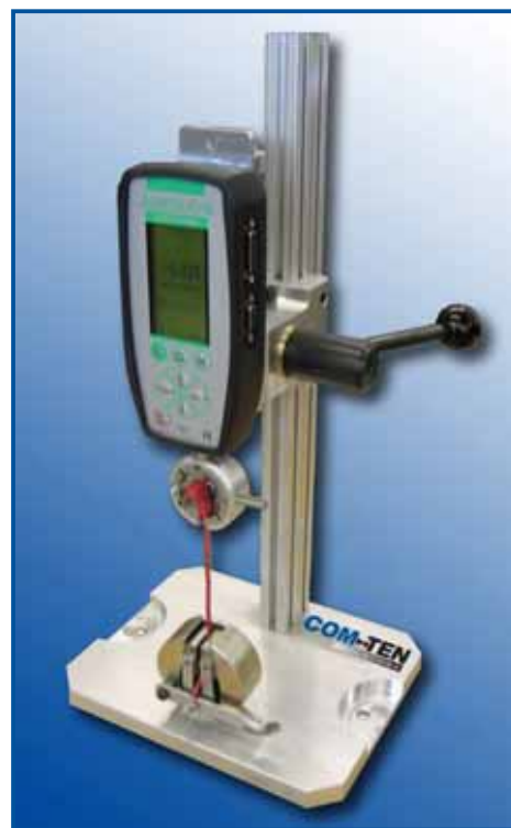
Tensile test on a wire with a TEX555 and a Centor Easy
