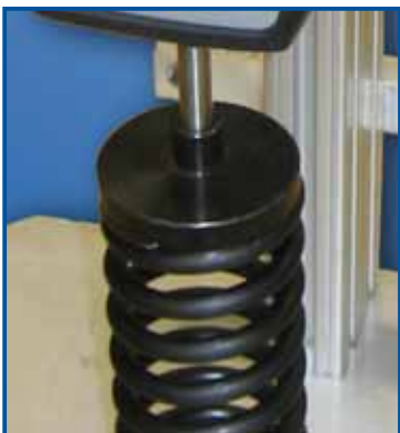
Compression test on a spring
