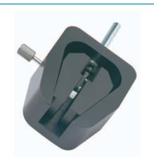
**Optional self-closing wedge clamp:** A self-closing wedge clamp cab replace the eccenrtic clamp when it is necessary. It is used to maintain wires, cables and terminals during tensile tests. Designed to increase the clamping force as the ten-sile force increases. It prevents any slipa-ge of the cable inside the grip. With a maximal opening of 0.2 in and a fast opening system, our self-closing wedge clamps can test easily all types of cables.
