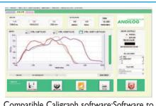
Compatible Caligraph software: Software to download curves on the computer throught RS232 or USB. Compatible RSIC software: download your results directly to Microsoft excel.
