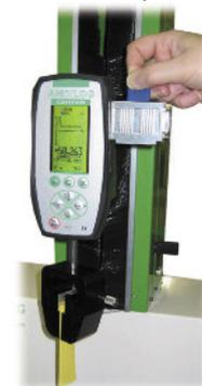
**Datastick Compatible:** SD memory card reader to save the values measured by the force gauge and then read them over on a computer for further processing.
