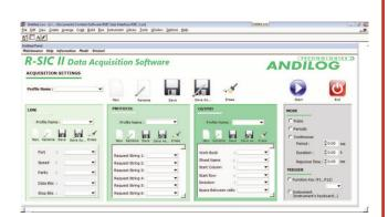
Compatible with RSIC software: saves your data on an Excel sheet directly through RS232. Allow real time communication as well as unloading the calculation values recorded in the Centor.
