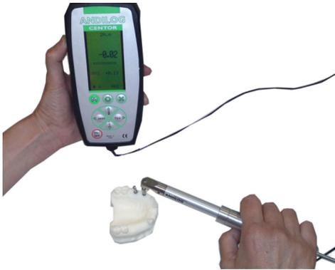
Developments in the medical industries also come with tools that measure the quality of medical parts (tools and aids) during the design, production, and installation process, or to track the life of implants. This is why ANDILOG has developed, in collaboration with laboratories, a torque measuring solution dedicated to research and manufacturers of prosthesis wishing to accurately measure the screw tightening torque of dental implants, and called the IMPLANTORK.
