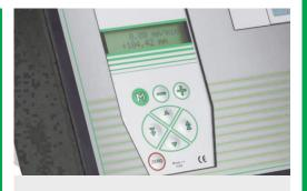
The manual motor command allows a smooth crosshead displacement to get into position before starting the measurements or to adjust first tests.
