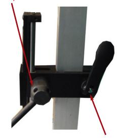
Adjusting the original height of the force gauge is done using the quick positioning cam handle, no tool is required.
