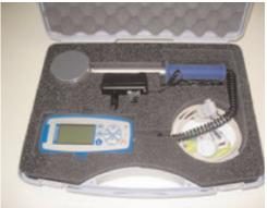
In compliance with the EN12456 and EN12445 standards, the ANDI-DOOR force tester instrument measures the closing force generated by automatic or power-operated gates, doors and barriers. As gate installers if you wish to comply with the machinery directive, you need to measure the impact force of the closing movement in the crush zones of the gates.
