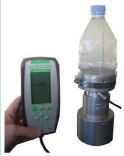
Instrumented bottle to measure the capping torque. The mechanical support includes the torque sensor and has been design according to the bottle shape
