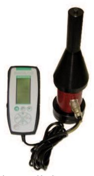
Instrumented bottle to measure the insertion force for champagne capping machine with a force sensor up to 2,000 lb
