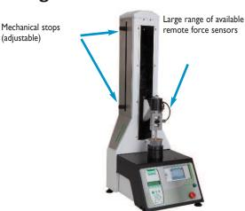
Large threaded working table to be used with different grips and fixtures
